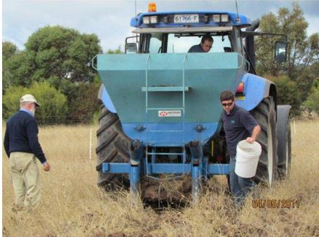
*The sub soil manure injector at work*
